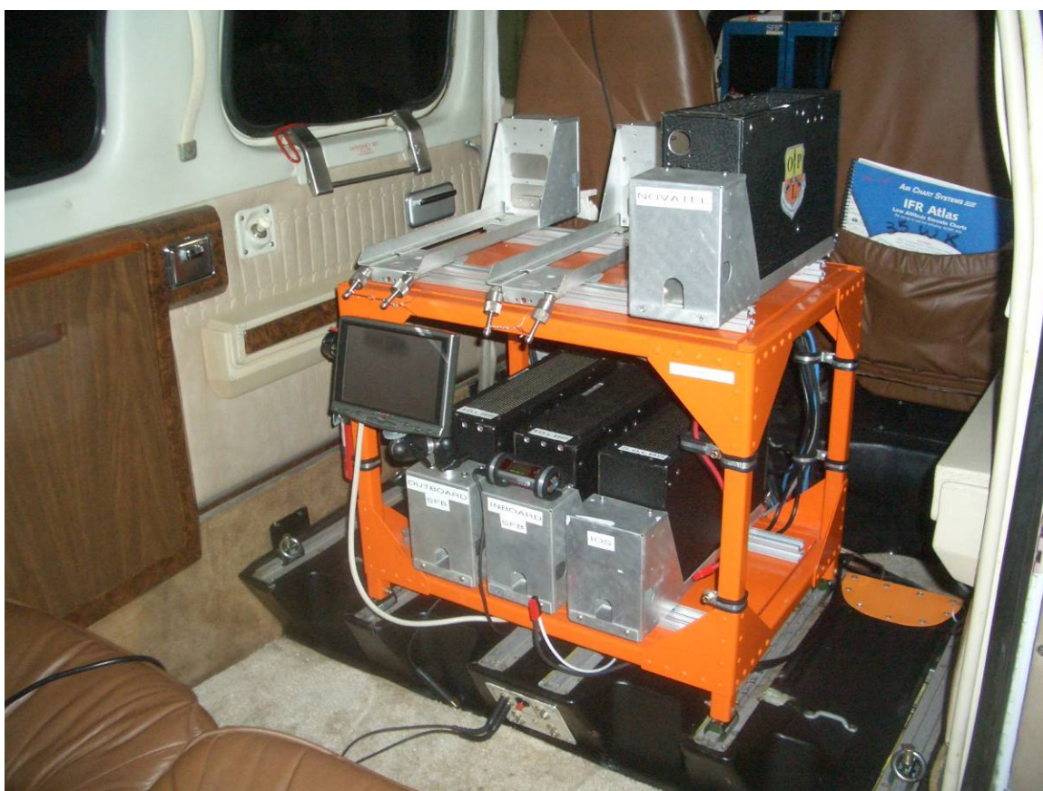
Figure 61 Equipment rack on the middle-row seat rails in the flight test aircraft.
