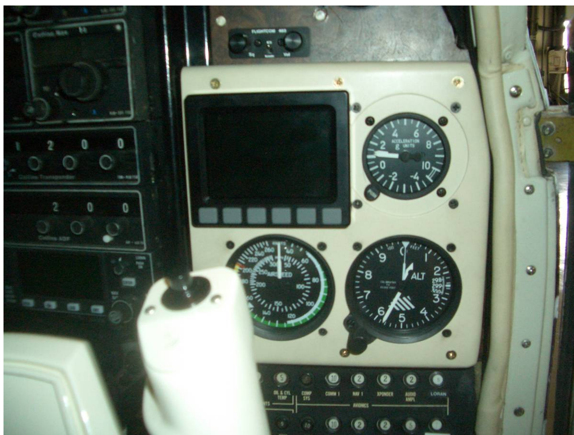
Figure 63 Supplemental instrument panel with Dynon EFIS-D10A installed.
