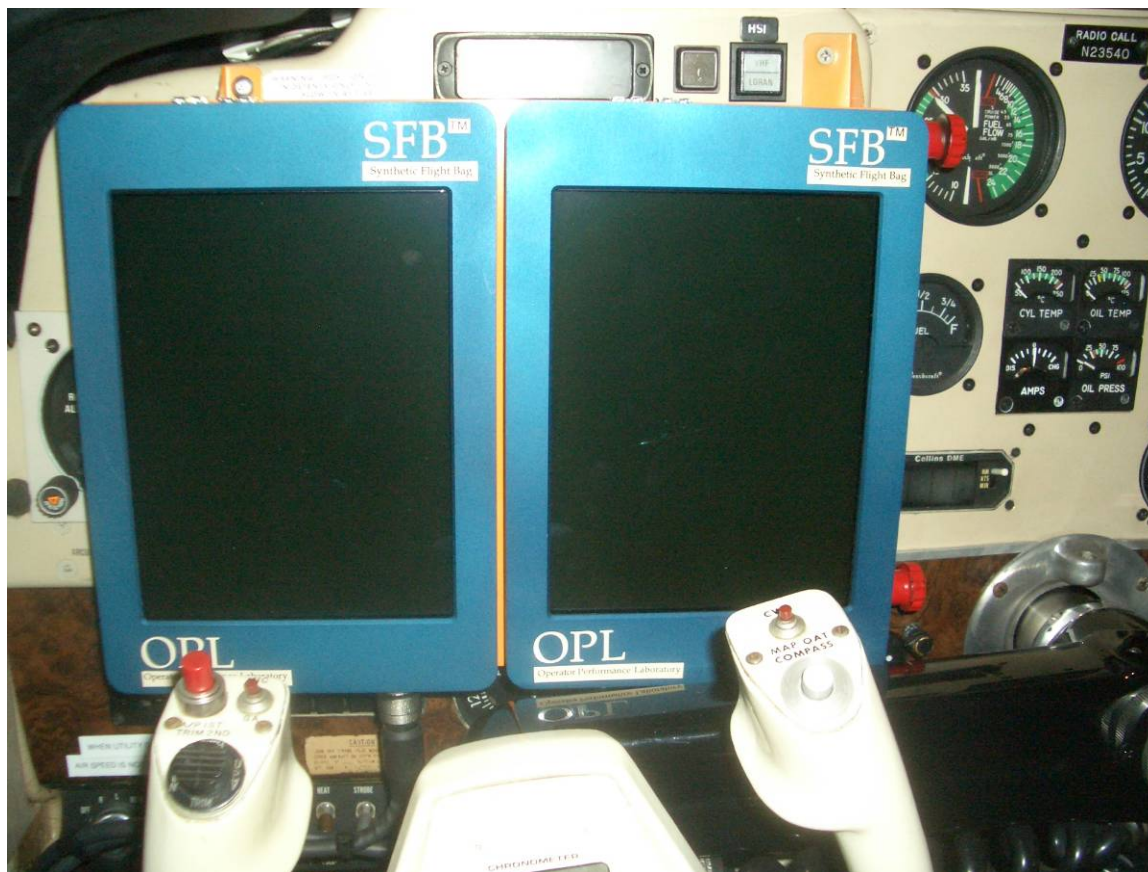
Figure 60 Pilot's instrument panel with dual-SFB displays installed
