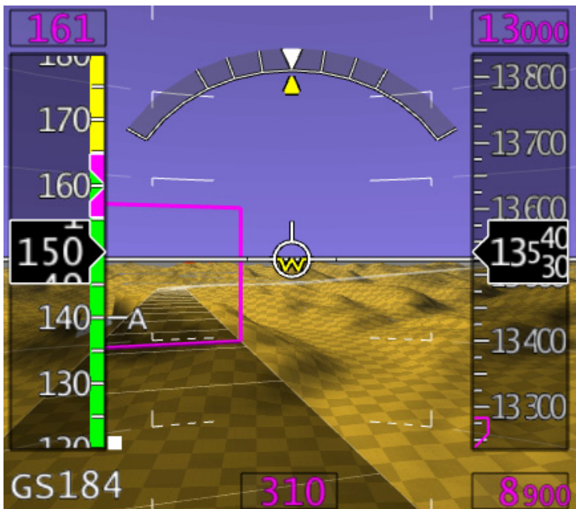
Figure 17 The SFB Primary Flight Display
